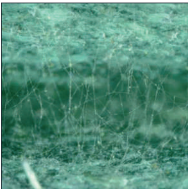
Fig. 7: Mould on test specimen 59 (H40), 40-fold enlargement.
