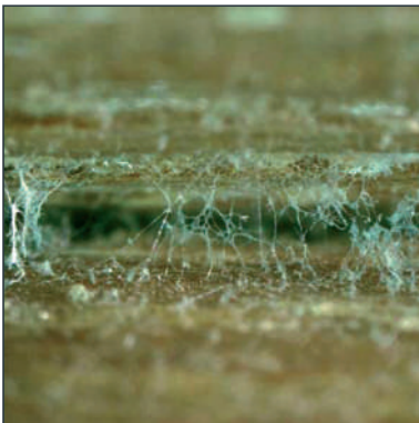
Fig. 9: Mould on test specimen 77 (Bangkirai), 50-fold enlargement.
